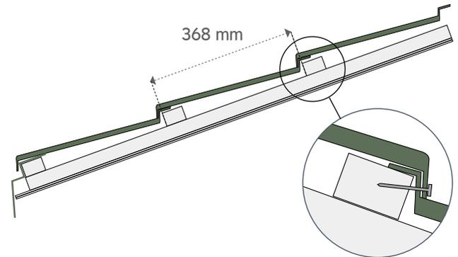
The panels are placed onto battens spacing 368 mm.
